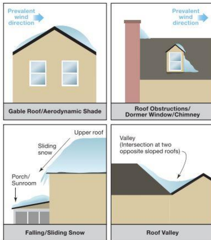
Figure 1a. Unbalanced snow load from drifting and sliding snow on typical commercial or industrial building
